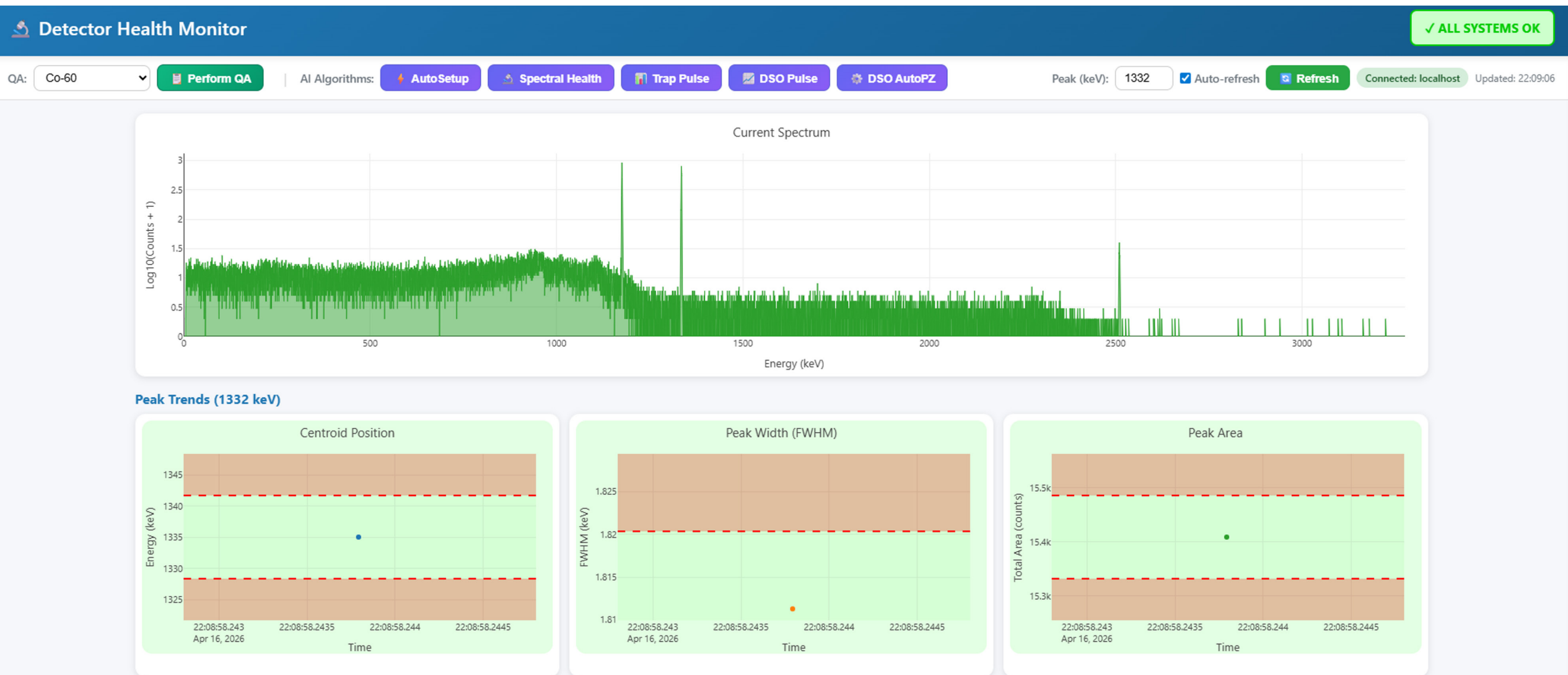
Figure 1 – Edge-Level QA & Predictive Maintenance Dashboard hosted on Lynx II. Accommodates easy QA checks and automatic Detector State-Of-Health monitoring, with AI optimization algorithms if a detector ever reaches QA limits.
