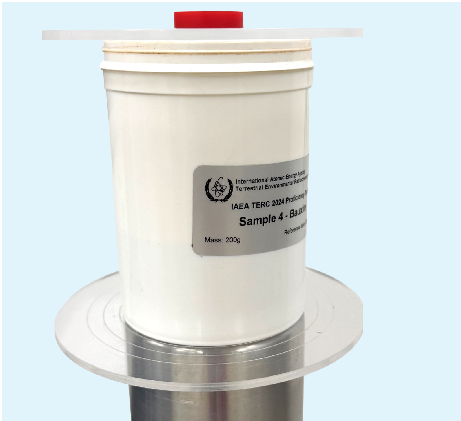
Schematic and photograph of the attenuation test. An Am-241/Eu-152 source is placed above the bauxite container. Gammas from the source must be attenuated by the bauxite, and thus the material properties of the bauxite may be inferred from the resulting spectrum.
