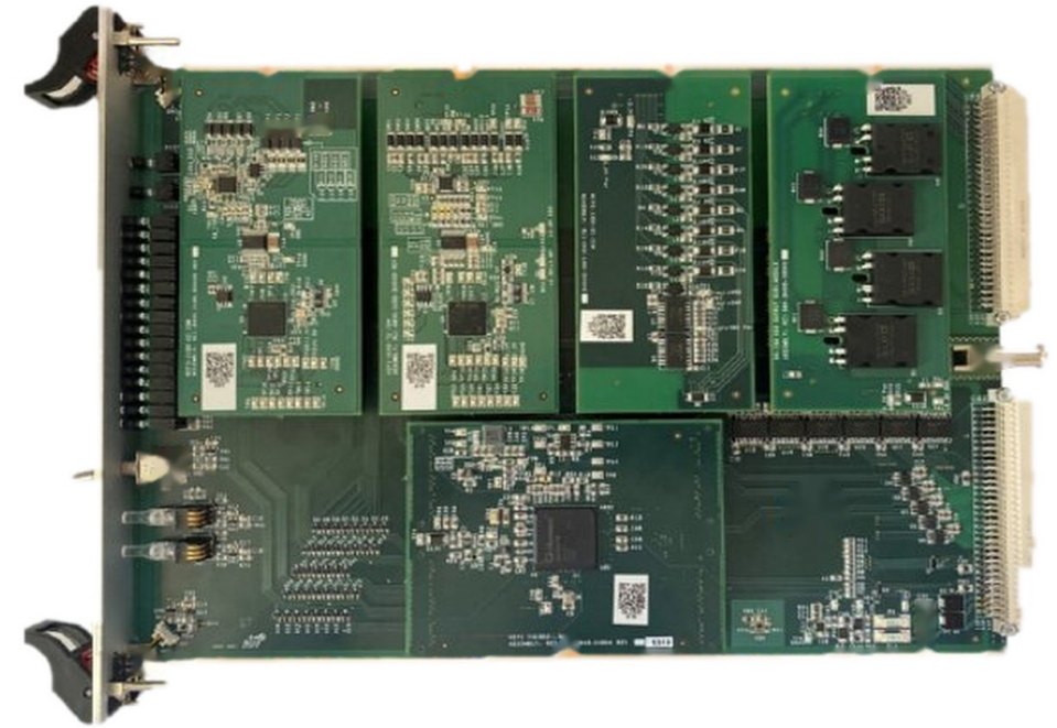
A HIPS module: UNO2 motherboard with logic and I/O submodules seated — handle one tonight at the Technology Hub.
