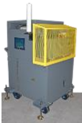
HPGe Primary Coolant Monitor
