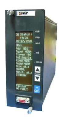
Power supply: 120 or 230 Vac Graphic display: 240 x 64 dots Visual alarm: 5 front LED Sound alarm: buzzer Upstream link 1 **Keypad: 3 push buttons** RAMSYS (RS485) Size: 5M x 5U Local RS232 serial link Upstream link 2 RAMSYS (RS485) isolated 8 isolated 8 isolated 5 relay 2 isolated (DPDT) digital analog analog digital
