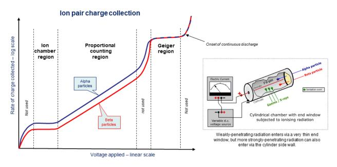
In the ion chamber region gas ionisation is direct and results in a current flow proportional to overall ionisation. At higher field strengths gas multiplication effects can be used, allowing output of individual ionisation events as measurable pulses.
