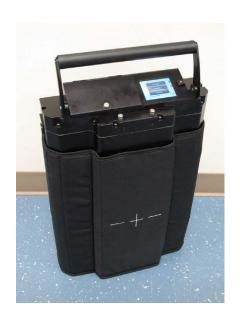
Portable, battery powered neutron counter
