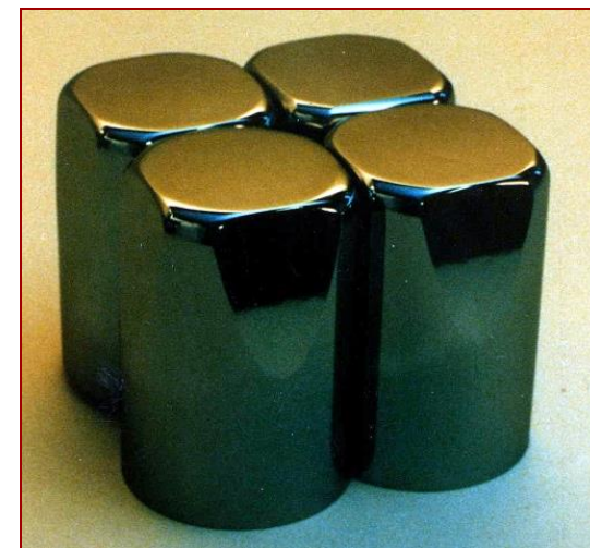
Compact arrangement of four coaxial Ge crystals in one single cryostat for large efficiency gamma spectroscopy.
