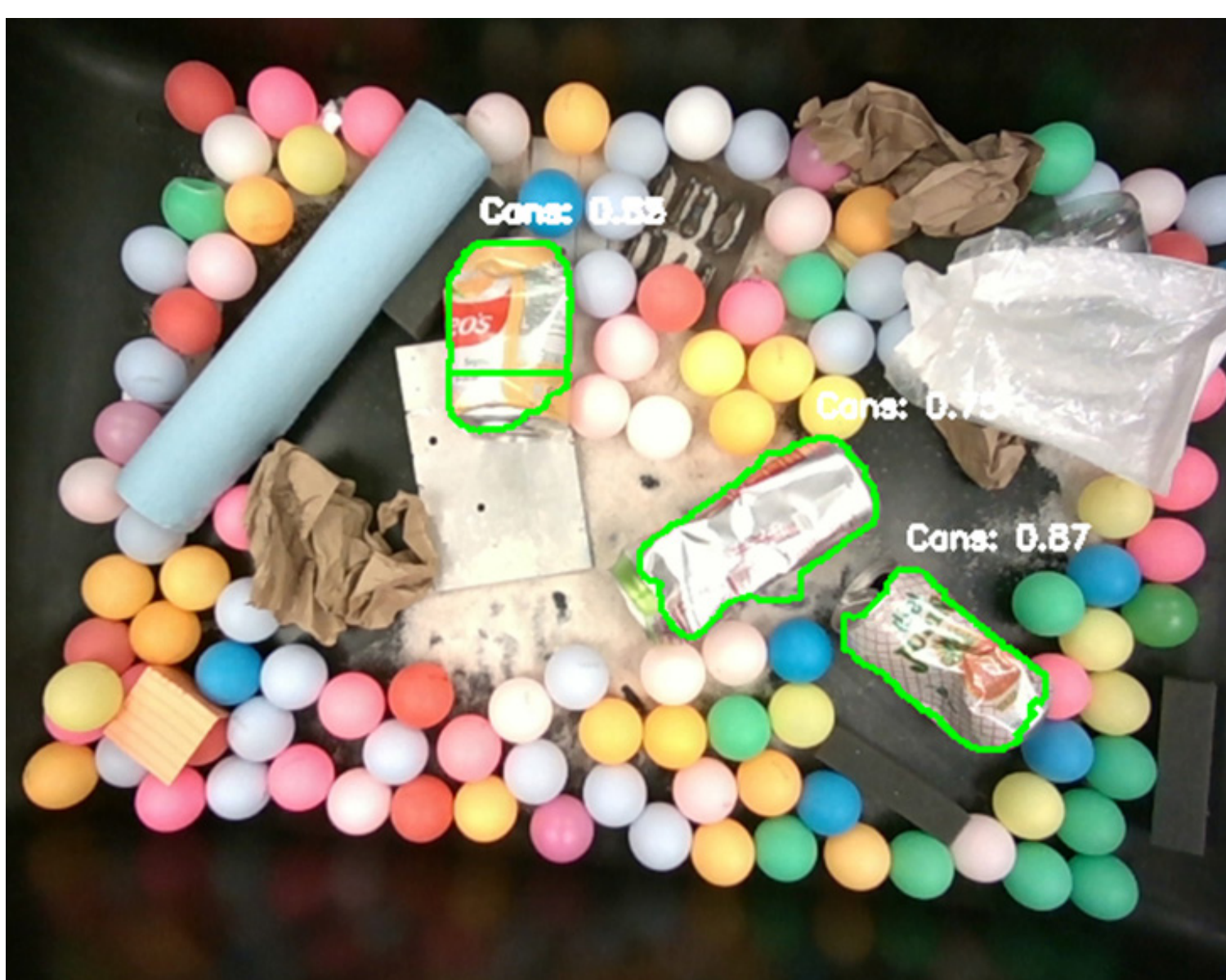
Figure 2. Object detection of soda cans using YOLO v8 with confidence level displayed
