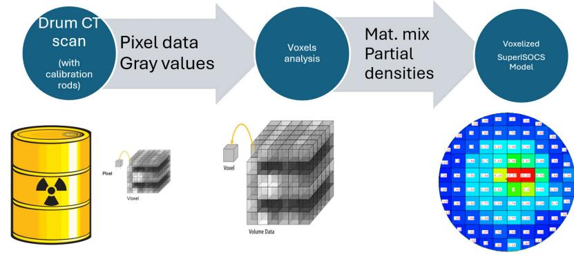
A 3D density map was then generated from the CT scan, integrated in a SuperISOCS template and used to simulate the detection efficiencies of the spectroscopy measurement.
