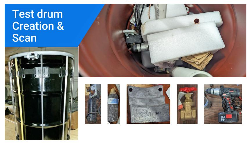
Rod sources of known materials (aluminum, copper, etc.) were positioned around the test drum for the X-ray scans in order to provide a base reference for the density evaluation process.
